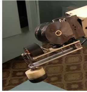
Fig. 6. Biomechatronic module with one-component force induction sensor
